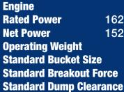
Cummins 6LT9.3 162 kW (217 hp / 220 ps) @ 2,000 rpm 152 kW (204 hp / 207 ps) @ 2,000 rpm 16,595 kg 3.0 m<sup>3</sup> rce 168 kN ance 3,037 mm
