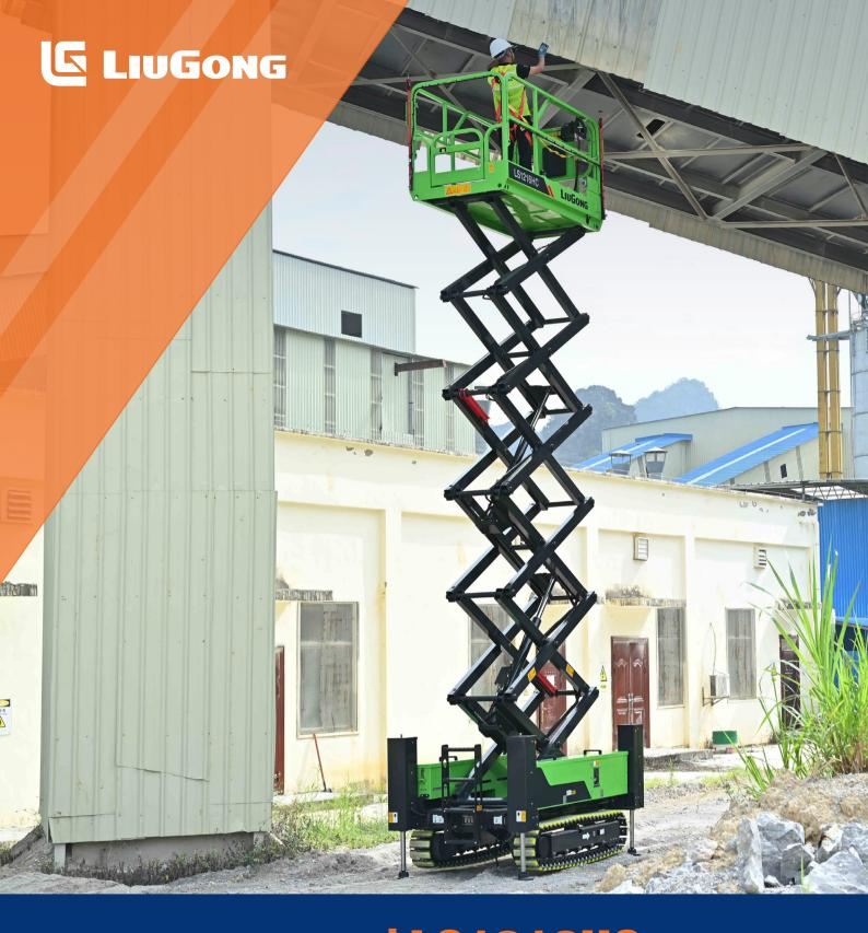
Working Height Max. Lift Capacity Max. Overall Width Overall Length Overall Weight 14 m (45'11") 320 kg (705 lb) 1.56 m (5'1") 2.8 m (9'2") 3,700 kg (8,157 lb)
